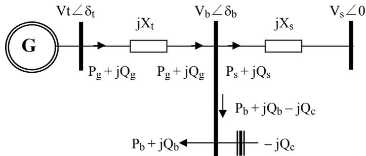
A-Fig. 4.1 1 machine, 1 load, and infinite bus model
