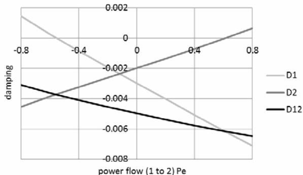
A-Fig. 1.4 Damping by tie-line flow (Cap. 2:3)
