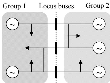
A-Fig. 1.1 Structure of inter area oscillation
