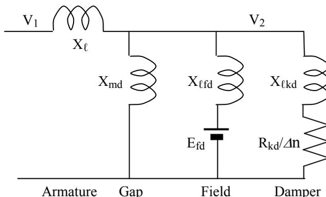
A-fig. 2.2 Equivalent circuit of direct axis
