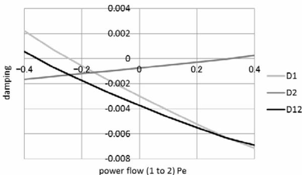
A-Fig. 1.5 Damping by tie-line flow (Cap. 1.4)
