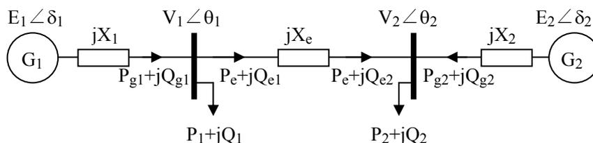
A-Fig. 1.2 Analysis model for inter area oscillation
