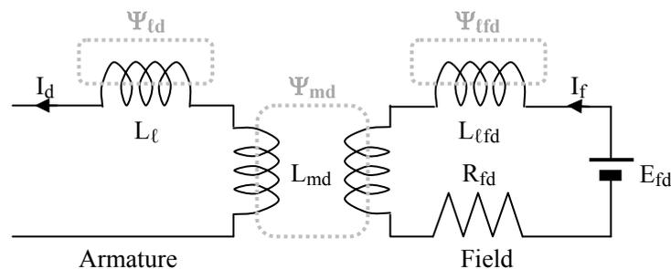
A-Fig. 2.1 Equivalent circuit of direct axis
