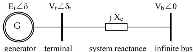
A-Fig. 3.1 1 machine and infinite bus model
