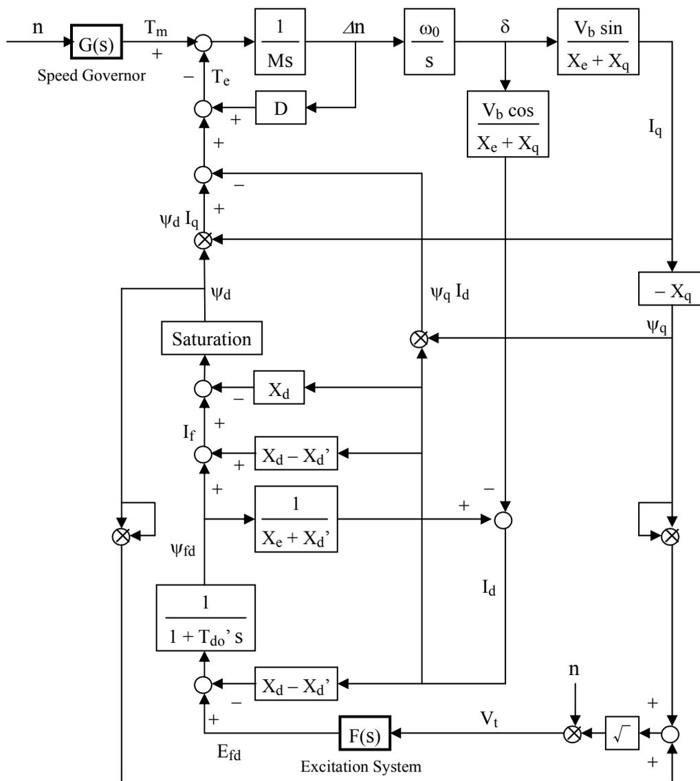
A-Fig. 3.3 Block diagram of 1 machine and infinite bus model
