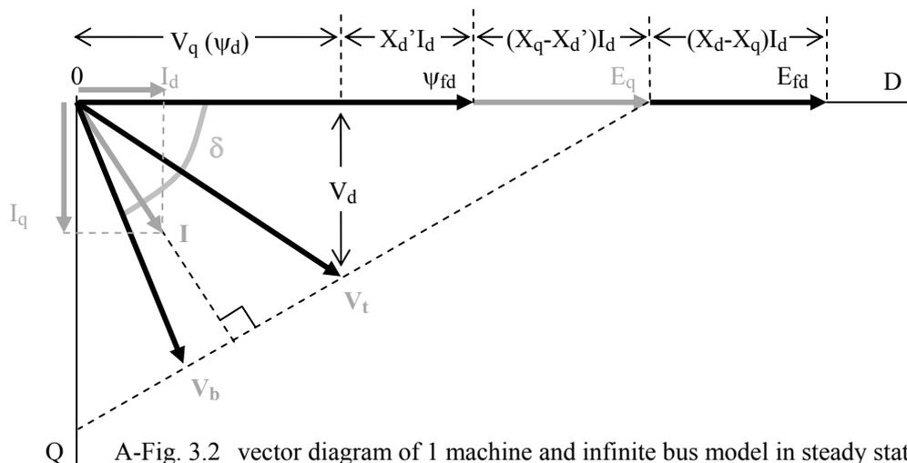
A-Fig. 3.2 vector diagram of 1 machine and infinite bus model in steady state
