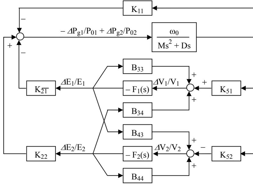
A-Fig. 1.3 Block diagram for calculating damping torque
