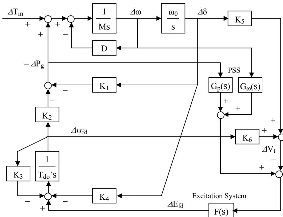
A-Fig. 4.2 Linearized block diagram of 1 machine, 1 load and infinite bus
