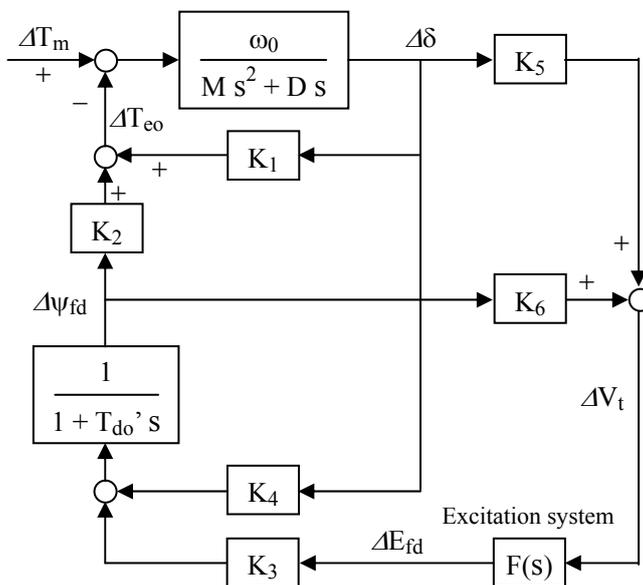
A-Fig. 3.4 Linearized block diagram
