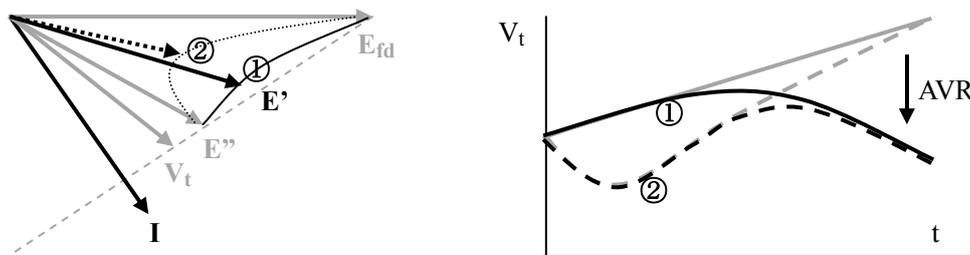
A-Fig. 2.3 Voltage profiles on disconnecting test by considering/ignoring  $X_q'$
